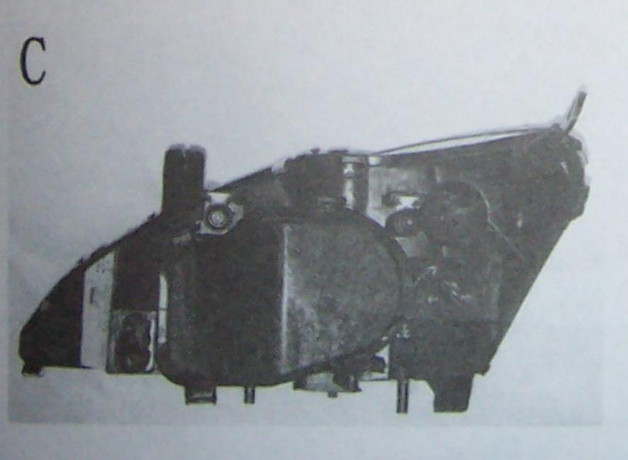
3. Picture (C) put the cover back after assembling the bulb.
